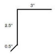
For custom eave drip, specify the amount of the eave that will be covered, and, for steeper roofs, specify pitch. If fascia is desired, specify the dimension you order will be concealed by the eave drip.
