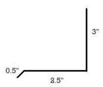
Like the ridge cap, the **ENDWALL** FLASHING can be sealed using outside closures. End-wall flashing is applied where the upward slope of a roof meets a wall. The wall side of the flashing can be covered with siding or counter-flashing, and outside closures are used to seal between the flashing and the panel. Roof slope should be specified when a roof slope exceeds 5/12 pitch.
