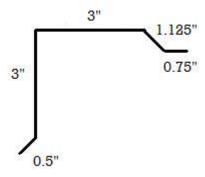
Gable flashing is used to trim the edge of the roofing panel at the gable end of the roof. It should match the eave drip extends along the drip edge of the roof. If the panel is allowed to hang over the gable end, eave drip can be used as an alternative. Butyl tape between the trim and panel eliminates potential leaks.
